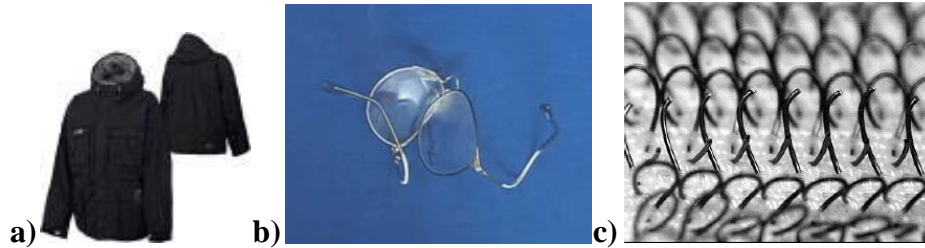
Figure 4.5: Phase changing materials in: a) textiles[3], b) glasses frames[2] , and c) thermal Velcro fasteners with clasps made from a nickel-titanium shape memory alloy [49]. [69]
